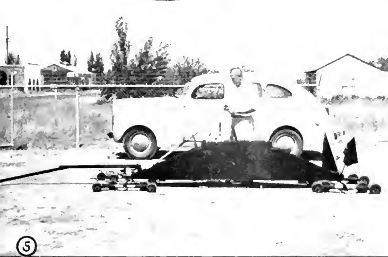
Units of profilograph machine for measuring pavement roughness. 2. Assembling the frame. 3. Close up of recording mechanism. 4. Plan view of the machine. 5. Profilograph assembled, ready for use. 6. Profilograph in use.
